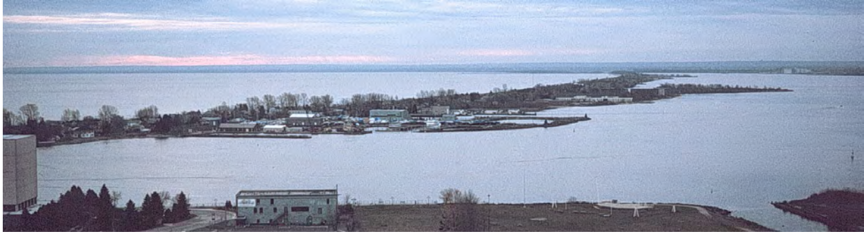
Figure I-2-21. Minnesota Point, photographed from Duluth, Minnesota, looking south (November 1994). This bay-mouth sand spit is reputed to be the largest fresh water barrier in the world. It extends from the Wisconsin shore near Superior to the Minnesota shore at Duluth. St. Louis Bay, to the right, needs regular dredging because of silt and sand supplied by the St. Louis River. The northern part of Minnesota Point is developed with residential property. Nearby Duluth and Superior are both major industrial centers, accessible by ocean-going ships
