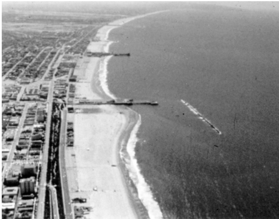
a. Salient with eroded downdrift (longshore drift is from bottom to top)
