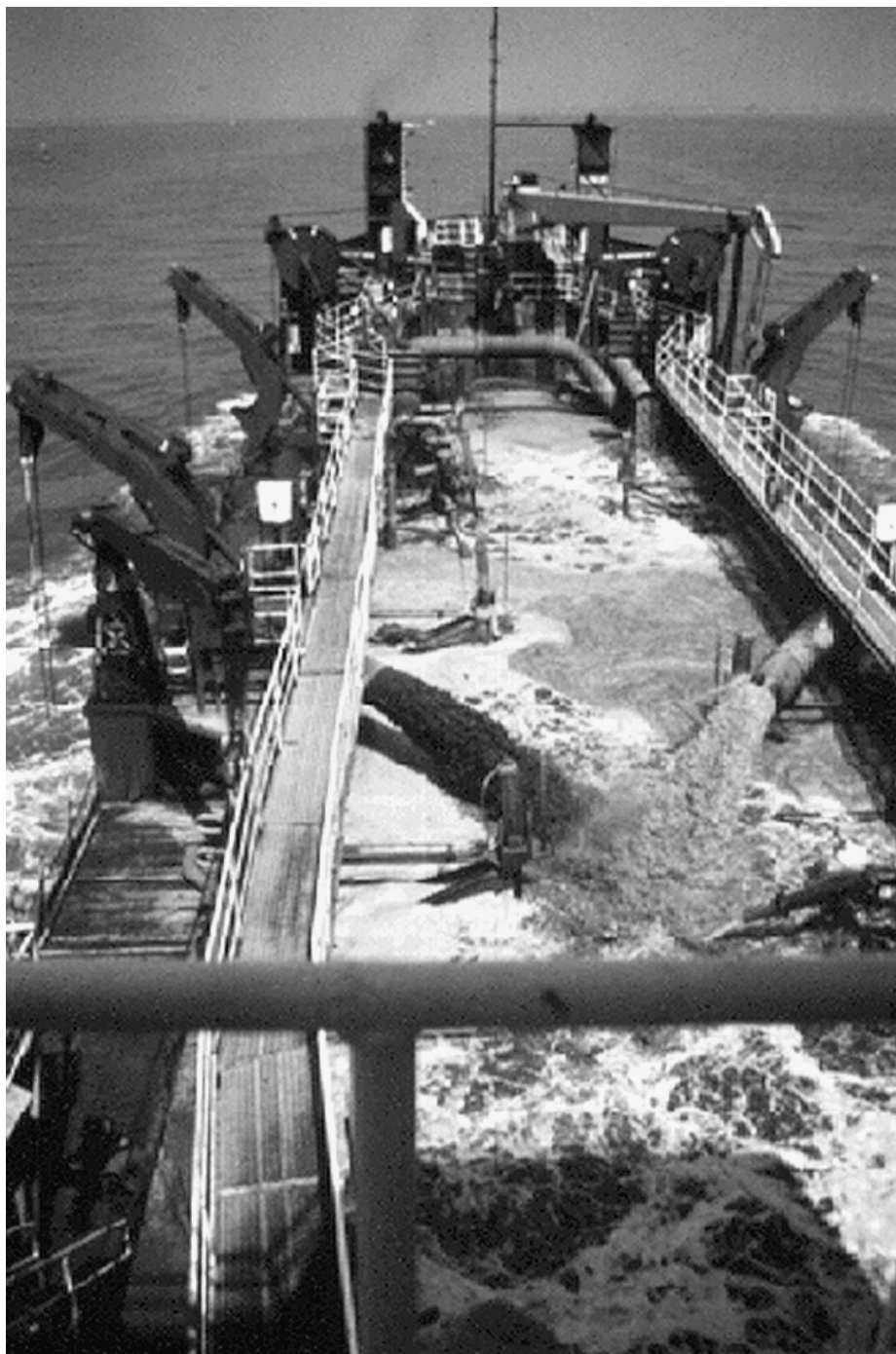
Figure V-6-61. Hopper dredge McFarland at Brunswick Harbor entrance, Georgia. Lightly colored sandy sediment (right-side intake) is mixed with dark colored silt and clay (left-side intake) during dredging
