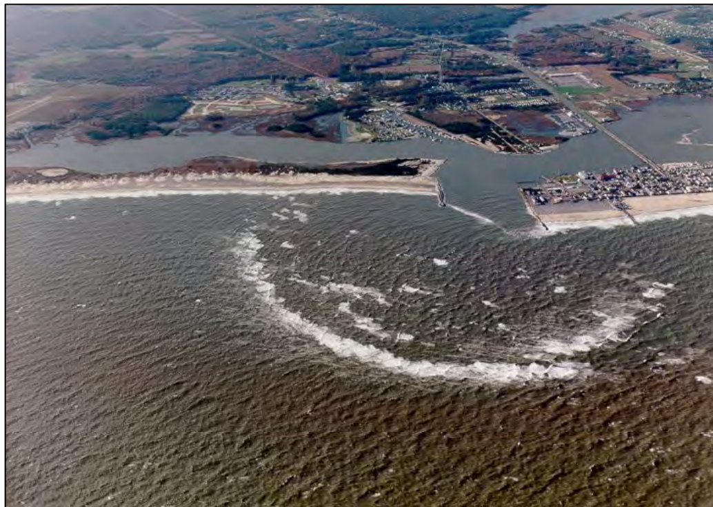
Figure V-6-40. Pattern of wave breaking on ebb shoal and bar, Ocean City Inlet, Maryland, November 1991
