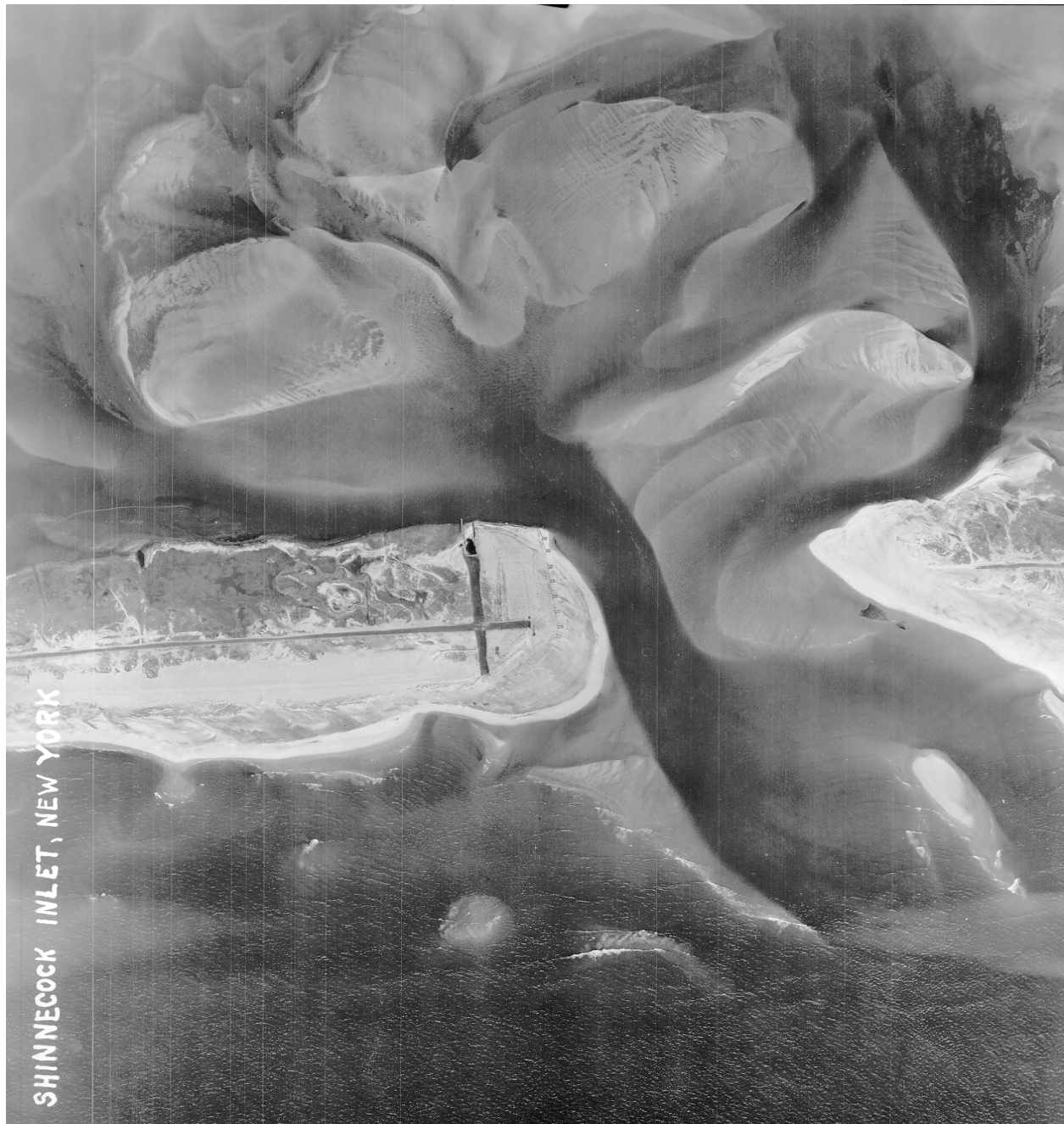
Figure IV-3-28. Shinnecock Inlet, New York, 1 April 1947. The inlet was much wider than in 1938, and a large flood shoal had accumulated. Some small shoals existed in the mouth of the inlet, but sediment transport had been largely directed into the bay since 1938. (Photograph from Beach Erosion Board archives)
