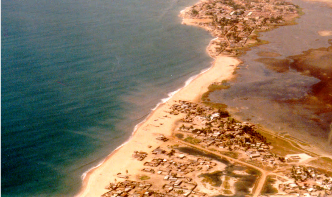
Figure III-5-5. Discolored water from erosion of exposed cohesive sediment along the Keta shoreline in Ghana, West Africa, July 1996
