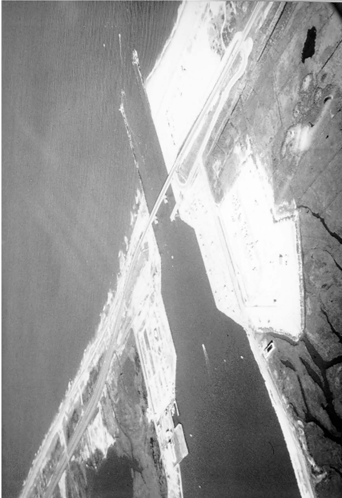
Figure III-2-1. Impoundment of longshore sediment transport at Indian River Inlet, Delaware
