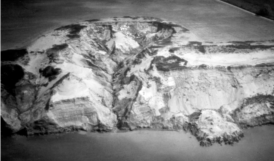
Figure III-5-22. Gully erosion of a bluff along the north central shore of Lake Erie
