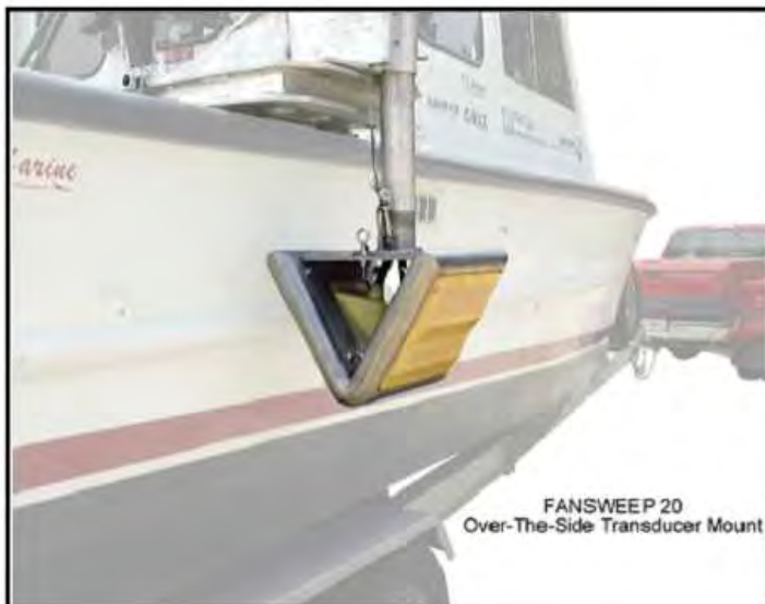
Figure 6-13. Typical multibeam transducer systems side-mounted on a rigid pole attached to the survey vessel. (Odom, Inc. and GeoAcoustics, Inc.)
