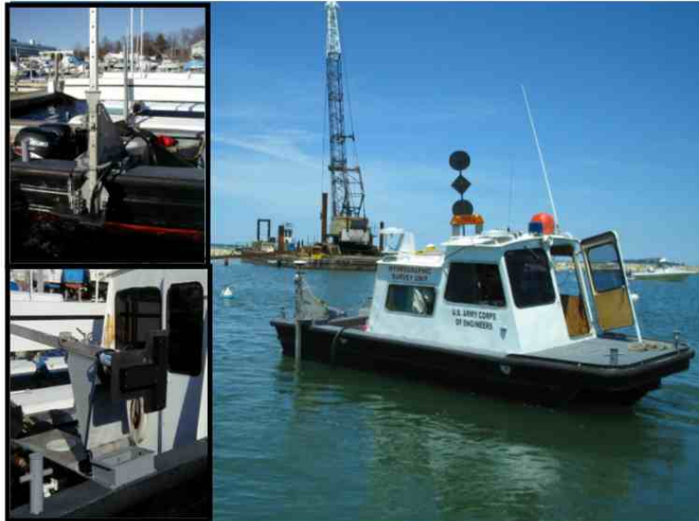
Figure 6-16. New England District survey boat with aft/side mounted multibeam system. The GPS positioning antenna is located directly over the multibeam transducer.
