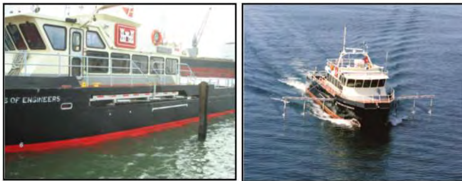
Figure 5-2. Survey Vessel Moritz Multiple Transducer Sweep System—54-ft swath with transducers spaced 6-ft c/c. Retractable boom fits flush with hull as shown in left photo. (New York District)
