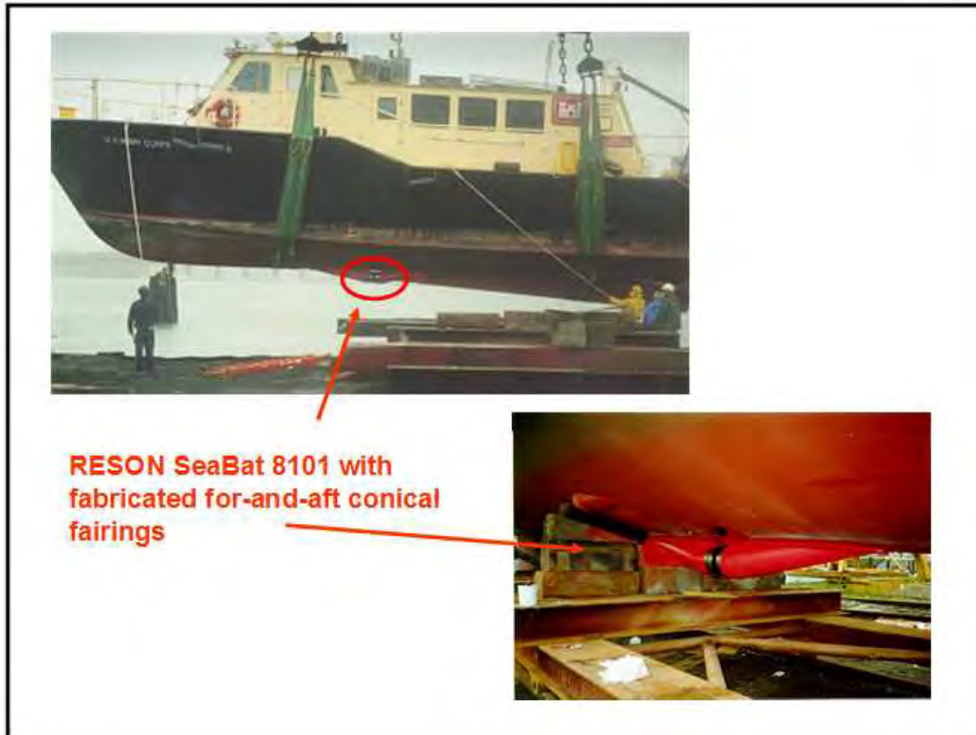
Figure 6-6. RESON SeaBat 8101 fixed hull-mounted installation on Survey Vessel Adams II. (1998 Norfolk District)
