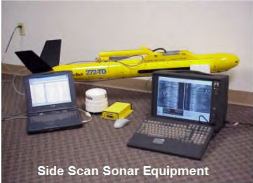
Figure Q-4. Digital side scan display system (Sea Systems Corporation)
