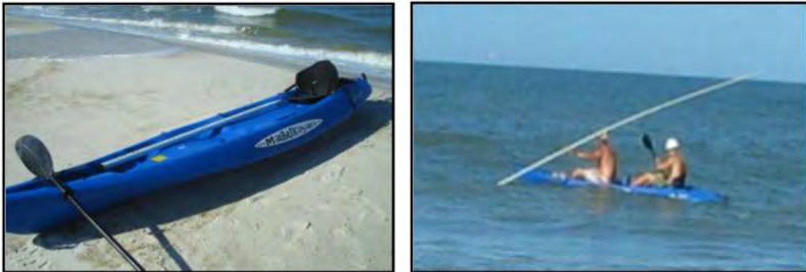
Figure 11-5. Kayak for obtaining deep water points just beyond wading range in Gulf of Mexico. Note that updated (2012) Corps policy requires surveyors to wear approved PFDs when working on a platform such as this.
