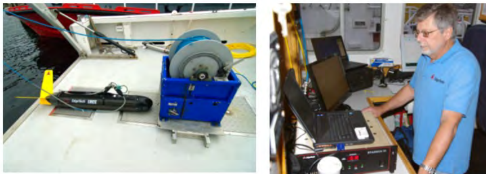
Figure Q-2. Basic components of a side scan sonar system. (left) Towfish and tow cable on winch. (Right) Sonar interface box and computer. (EdgeTech)
