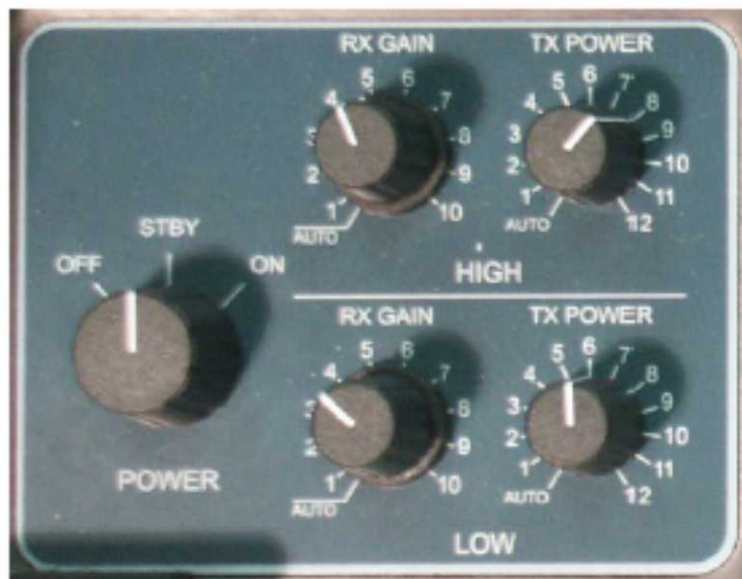
Figure 4-4. Odom MKIII transmit (TX Power) and receive power (RX Gain) adjustments. Maintaining consistency in these adjustment settings is critical in ensuring survey repeatability in soft material.
