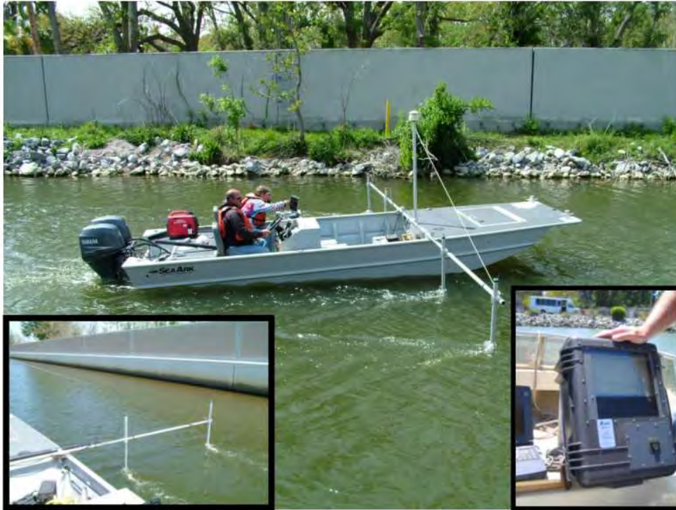
Figure 5-7. Ross 875-4 sweep system surveying the London Avenue Canal in New Orleans, LA, after Hurricane Katrina (2005). (St. Louis District)
