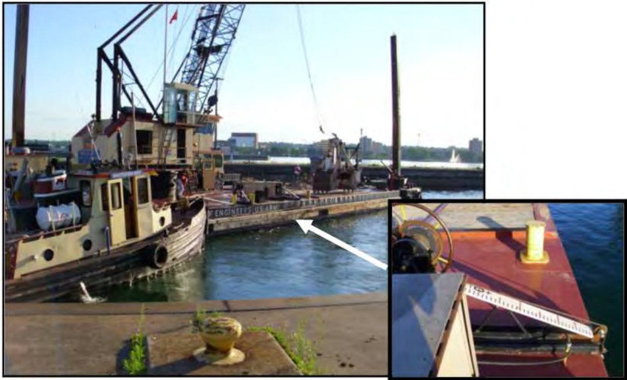
Figure 10-6. Detroit District Derrick Barge Nicolet. The barge deploys both a single bar sweep and a multibeam system to aid in object detection and removal.
