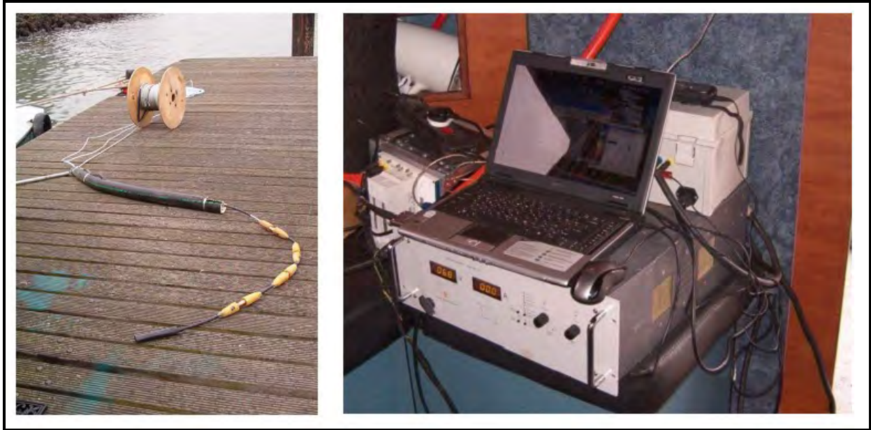
Figure P-16. Rheocable Method towed array and deck unit.
