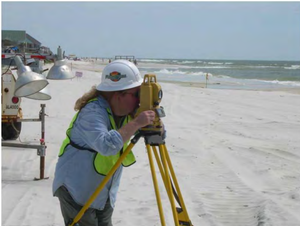
Figure 11-6. Total station control of topographic beach profiles.
