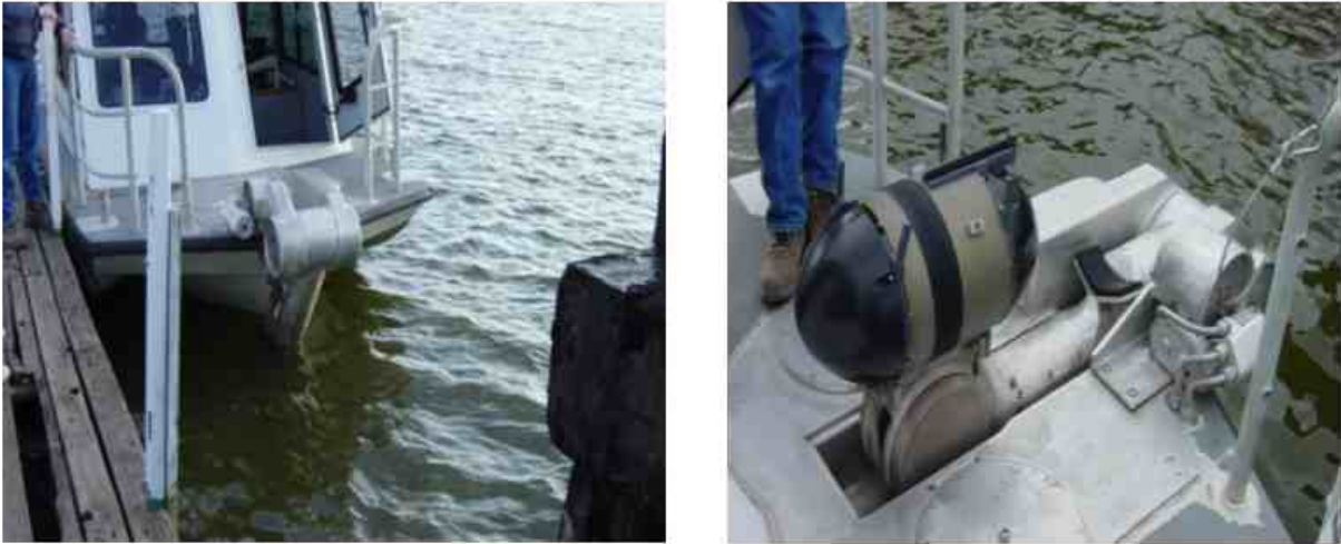
Figure 6-10. Tulsa District retractable bow-mount. It is hydraulically deployed.
