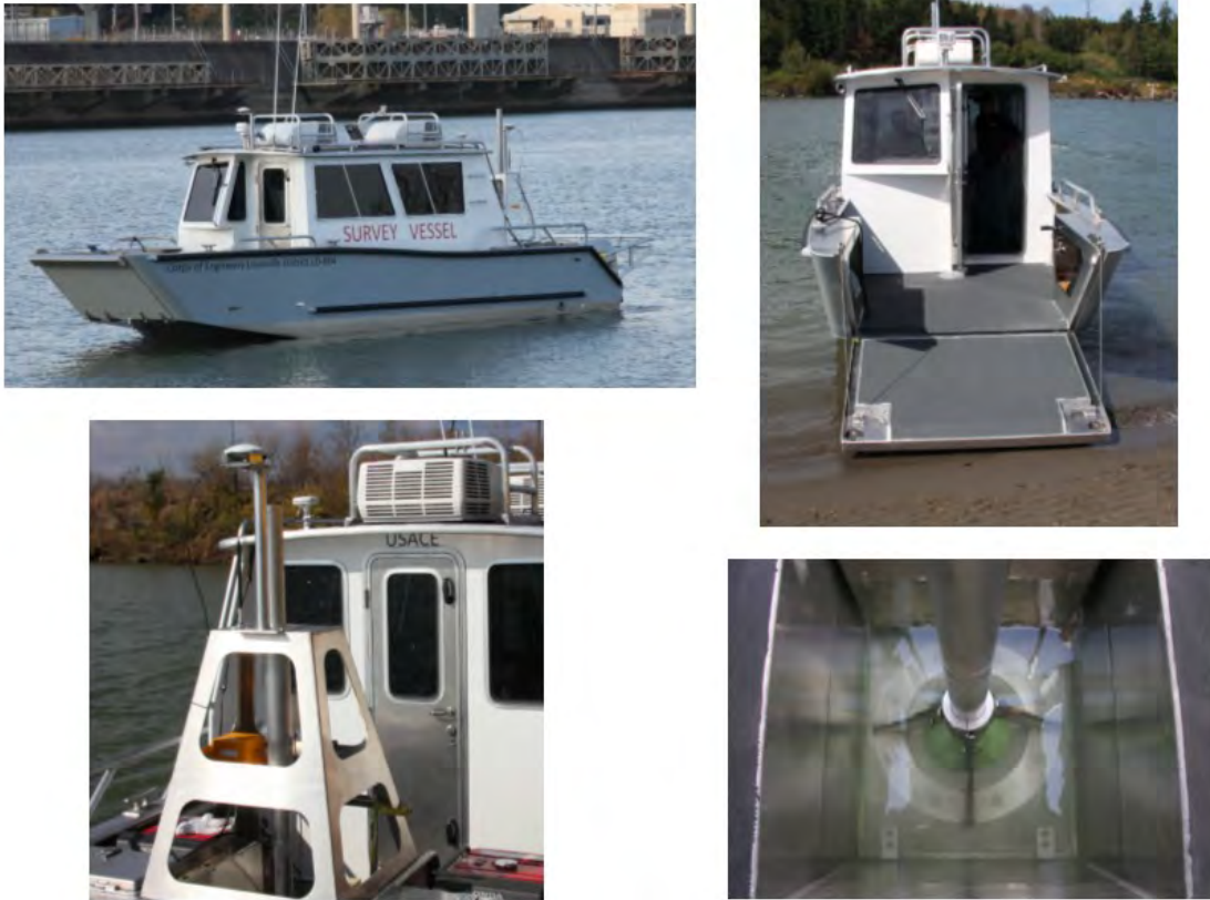
Figure 6-8. Louisville District 30-ft survey boat with through hull mounted transducer (Reson 8125-H multibeam system).
