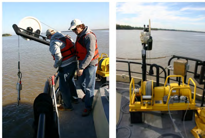
Figure P-20. Rheotune probe being deployed off the New Orleans District S/V Teche via a semi-automated winch.
