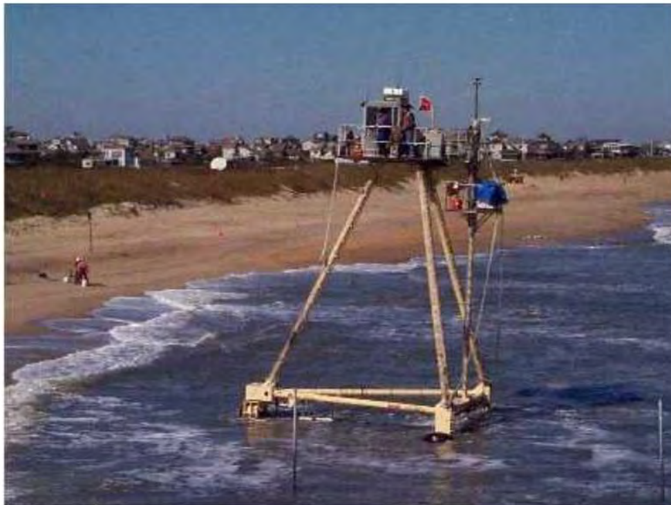
Figure 11-7. CRAB. Hydrographic survey platform used for research purposes by the ERDC Coastal and Hydraulics Laboratory research facility at Duck, NC. (ca 1980s)
