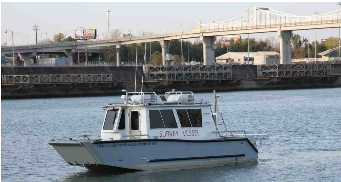
Figure N-12. Louisville District 30-ft multibeam survey boat. This vessel is typical of those used for investigation surveys around Ohio River locks and dams. The Reson 8125 transducer is deployed through a moon pool in the hull.
