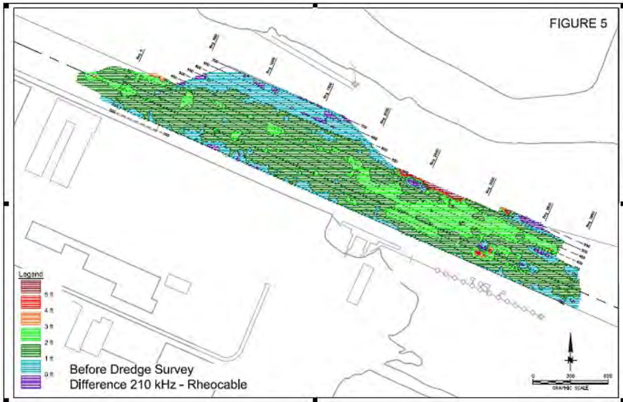
Figure P-18. Difference plot between Rheocable and 33-kHz depth measurements demonstrated in Wilmington Harbor, DE.
