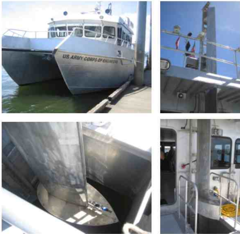
Figure 6-7. Portland District S/V Redlinger. The S/V Redlinger is a 60-ft foil supported catamaran. Survey equipment includes an Applanix POS/MV, Simrad EM 3002, and an Odom CV100. The transducer is located just aft of the cabin.
