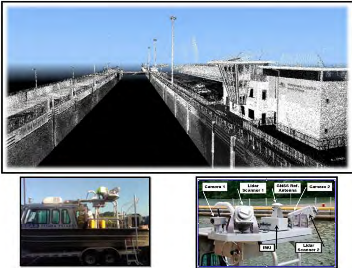
Figure N-21. OPTECH LYNX marine mounted laser scan of Marmet Lock & Dam, Kanawha River, Huntington District. (Seaside Engineering and Surveying, Inc.)
