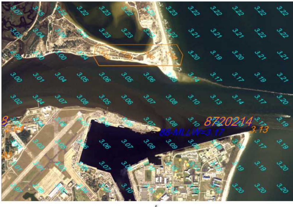
Figure 7-6. Example of a KTD file generated from VDatum. (Ocean entrance to Mayport Naval Base, St. Johns River, FL). “K” values are “NAVD88 – MLLW.” Note incorrect VDatum and KTD interpolation on north side of entrance, between the river and tidal pool. This region required manual edits to the KTD file to correct. Published NOAA gage 8720214 “K” at South Jetty agrees closely with VDatum “K.”
